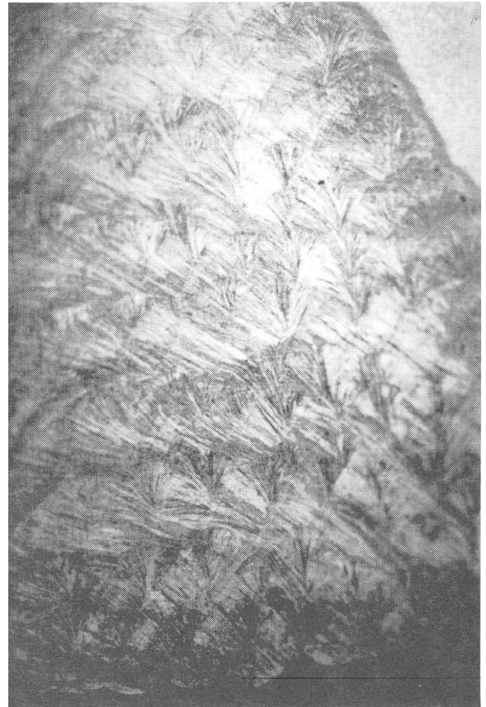
Fig. 6. Dendritic crystalline formation on a polished and etched full penetration weld on a thick flange.
